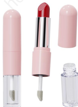
PH137B1 | Size: \Phi 20.80 \times H109.54 mm Capacity: 5.5ml Bottle: OFC/3.7ml NFC/2.4ml Cap Materials: PP/3g Midsection Materials: PP/2.9g Rod Materials: PBT/1.8g Wiper Materials: LDPE/0.4g Brush Materials: TPEE/TPU/0.2g Bottle Materials: PETG/11.3g
