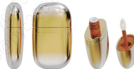
PH128B1 Size: L43.22*W20.92*H72.02mm Filling: OFC/4.4ml NFC/3.0ml OUTER COVER Materials: ABS /3.7g INNER COVER Materials: PBT /3.1g FLOCKED TIP: Share PH117UA WIPER Materials: LDPE / 0.3g NECK Materials: PETG / 3.9g INNER SHELL Materials: PETG / 2.5g OUTER SHELL Materials: PETG / 13.6g
