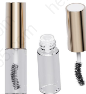
XJ651D1 Size: Ø18.00*H76.30mm Bottle: Ø18.00*H49.50mm Capacity: 7.7ml/OFC 6.0ml/NFC Wiper Materials: LDPE/0.4g Bottle Materials: PETG/4.4g Top Materials: ABS/0.7g Cap Materials: ABS/3.4g Stem Materials: PBT/1.3g Thread Spec: 14.30mm/T 11.00mm/H
