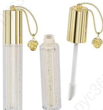
PH123B1 Size:L19.62*W19.13*H103.70mm Filling:OFC/6.0ml NFC/4.8ml Wiper Materials: LDPE/0.2g Top Materials: PP/0.2g Collar Materials: PETG/0.2g Cap Materials: PETG/3.8g Bottle Materials: PP/2.0g Stem Materials: POM/2.0g Base Materials: PETG/7.3g Brush Materials:Share PH123VA
