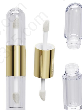
PH144B1 Size: Ø20.42*H104.68mm Bottle-1: OFC/3.7ml NFC/2.4ml Bottle-1: OFC/3.7ml NFC/2.3ml Bottle-1 Materials: PETG/12.3g Bottle-2 Materials: PETG/11.3g Brush Materials: TPEE/TPU/0.2g x2pcs Rod Materials: PBT/1.8g x2pcs Wiper Materials: LDPE/0.4g x2pcs Midsection Materials: PP/2.9g
