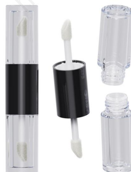
PH144A1 Size: Ø20.80*H111.31mm Bottle: OFC/3.7ml x2pcs NFC/2.4ml x2pcs Bottle Materials: PETG/11.3g x2pcs Brush Materials: TPEE/TPU/0.2g x2pcs Rod Materials: PBT/1.8g x2pcs Wiper Materials: LDPE/0.4g x2pcs Midsection Materials: PP/2.9g
