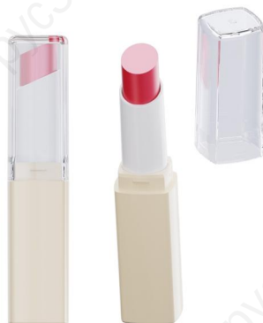
B184A1 | Size: L18.68*W18.68*H87.90mm Cup: \Phi 11.20 mm Filling: 3.5ml (Top Fill) Cover Materials: PETG/5.3g Shell Materials: PP/1.6g Cup Materials: POM/1.4g Screw Materials: POM/1.3g Weight Materials: 4.5g Bottle Materials: PETG/9.8g
